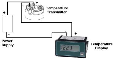
Redrawing the circuit above we can see how to wire into a junction box:
