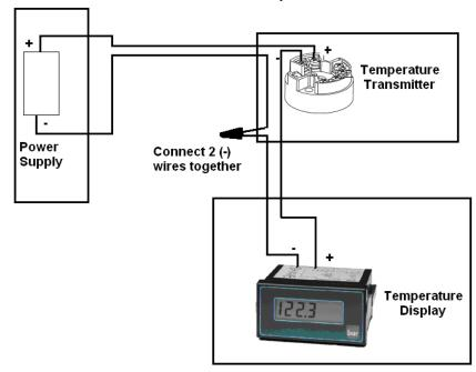
**What if I need a PLC input?** This is a common question. To add a PLC or computer input, just insert it in the loop. Remember  $(+) \rightarrow (-)$ ,  $(-) \rightarrow (+)$  except at the power supply.
